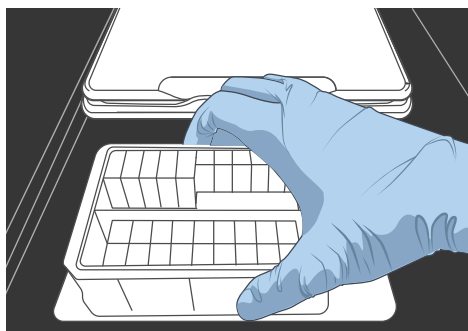
Figure 8 Placing DNB Load Plate
