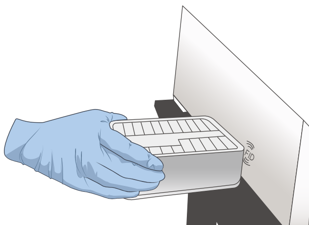
Figure 30 RFID scanning area of DNB Load Plate
