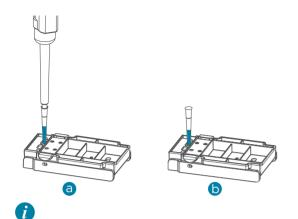
Do not touch or move the tip when ejecting the tip. Failure to do so might bring bubbles into the flow cell.
